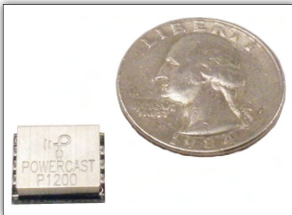
Powerharvester Module P1200 pictured with U.S. quarter to demonstrate size ratio.
