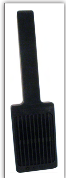
Fixed Antenna Powercaster Module
